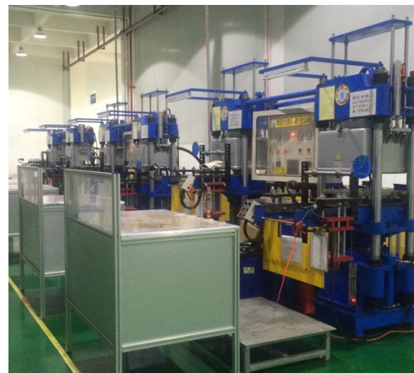
橡胶硫化模压机 Mould Pressing machine
