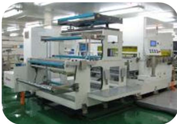
1200mm*1000mm Die cutting machine 大尺寸光学模切设备
