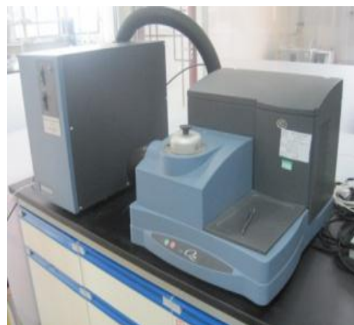
DSC差示扫描量热仪 Differential Scanning Calorimeter
