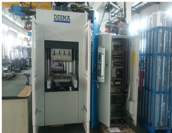
DESMA 橡胶注射机 Inject machine
